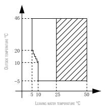
Water flow temperature drop or rise interval
