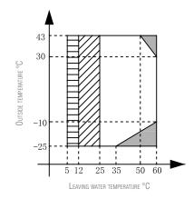
Water flow temperature drop or rise interval
