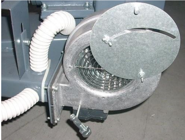
Picture 11. The position of the flap of fan
