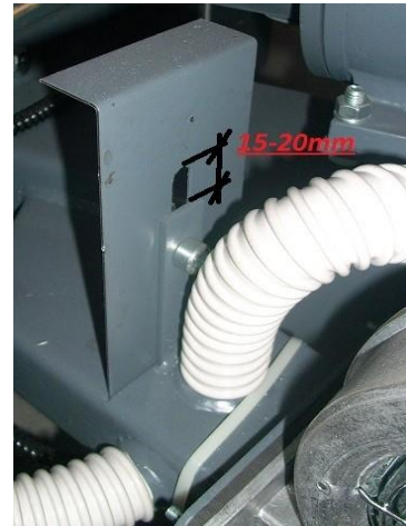
Picture 12. The position of the completely open flap of the fan
