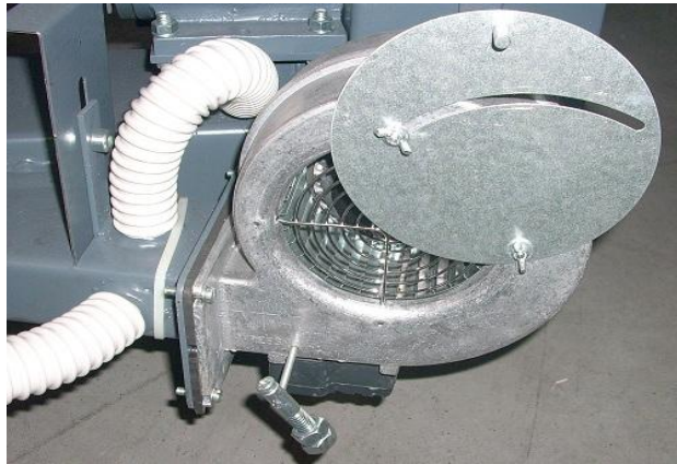
Figure 13. Position max. open of the fan flap
